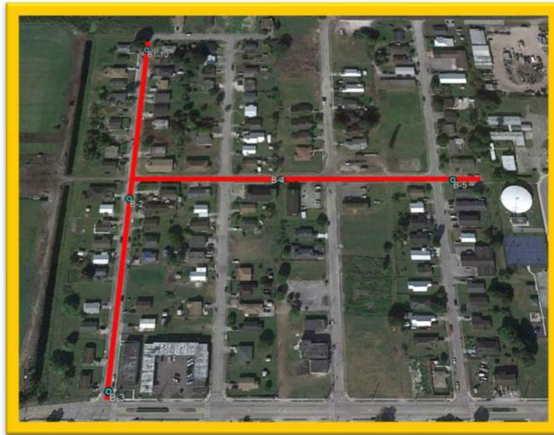
FIGURE-3: PROPOSED BORING LOCATION PLAN
